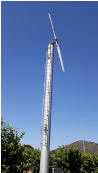
Wind machines help keep the lemon and avocado trees from freezing
